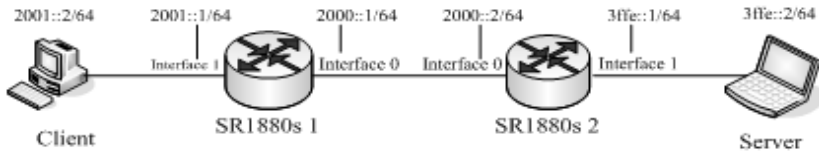
Fig. 9. Architecture of Testing Security Module with Two Routers
