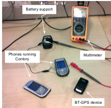
Fig. 3. Power measurements testbed setup
