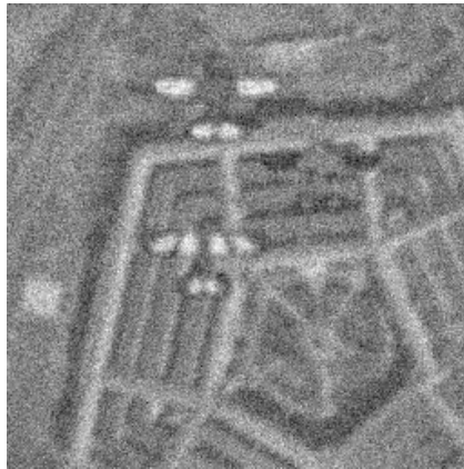
Fig. 2. Observed image with a uniform PSF (size d=5 ) and AWGN with \mu_n=0 and \sigma_n=20
