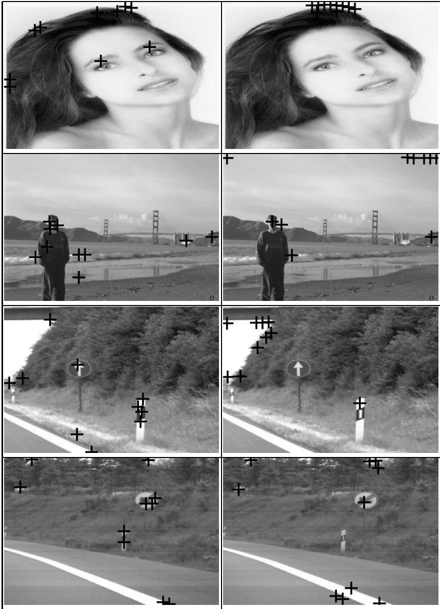
Fig. 5. Results of the attention mechanism with optimized (1st column) and standard (2nd column) weights on test images available at http://ilab.usc.edu/imgdbs/
