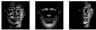
Fig. 4. The first image is the original needle map projected to the x direction of the viewing plane. The second image is the mean needle map that we use as the template. The third image is the needle map projected to the x direction of the viewing plane after the Mean Needle Map Alignment (Sect. 2). The third image compensates the concave/convex problem of the first one.
