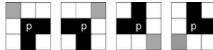
Fig. 2. Masks for final thinning. Black squares and gray squares denote skeletal pixels and background pixels, respectively. White squares are don't care pixels, but among them at least one edge-neighbor of p in each mask must belong to the background.
