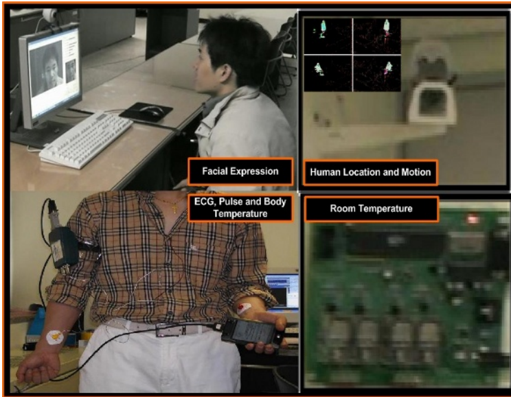
Fig. 2. Four sensor devices for extraction of seven contexts
