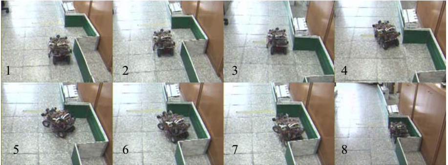
Fig. 6. Experimental results of the parallel-parking control
