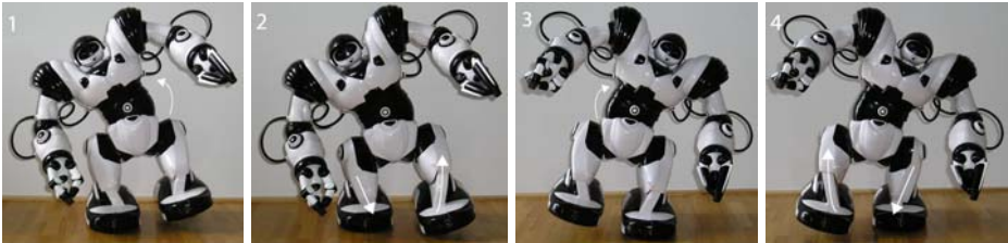
Fig. 2. Dynamic walking gait of RoboSapien. (1) The trunk motor tilts the upper body to the right. The center of mass shifts over the right foot. The left foot lifts from the ground. (2) The leg motors move into opposite directions, resulting in a forward motion of the robot. As the upper body swings back, the left foot regains contact with the ground. (3,4) Symmetrical to (1,2).
