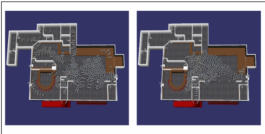
Fig. 4. The image on the left is the evacuation visualization at 5 seconds; the image on the right is the evacuation visualization at 30 seconds. The Case 1 visualization is shown
