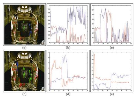
Fig. 2. 3D-from-2D motion segmentation. (a) shows a picture with 76 points over four separate bodies, (b,c) show the resulting four columns of the partition matrix G using SNTF with a 9-way affinity array. The bottom row shows the results after projecting the affinity array onto a matrix. The projection resulted in significant information-loss which caused performance degradation.
