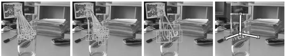
Fig. 7. Detecting a transparent object with partial texture. The squares in the first three images outline the patches around the features detected at three different scales in a test frame. The straight line segments connect the feature with the corresponding one in a frame of the training sequence. Since during training the system learned which parts of the patches are meaningful as shown in Fig. 3, the image features can be recognized even if the patch overlaps the background or the transparent parts. As shown in the fourth frame, the glass is successfully detected.
