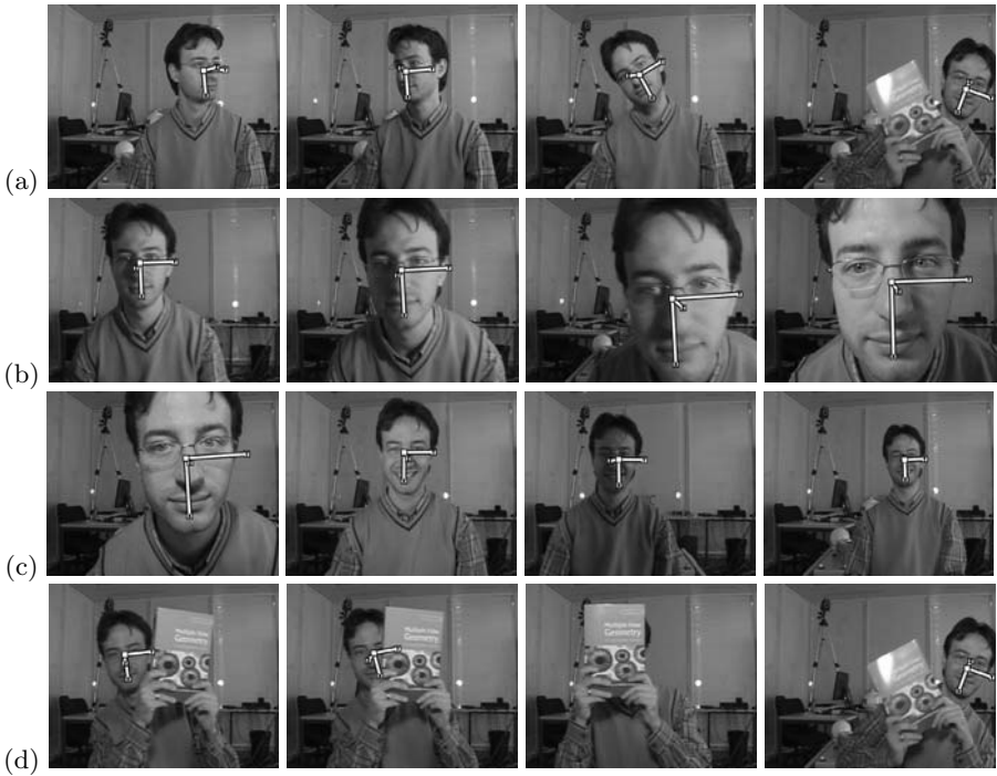
Fig. 6. Face results. Note that by contrast with previous face detection approaches, the face pose can be retrieved under (a) large rotations, (b) scale and lighting changes, and (c) different facial expressions. (d) After the occlusion by the book, the algorithm automatically recovers.
