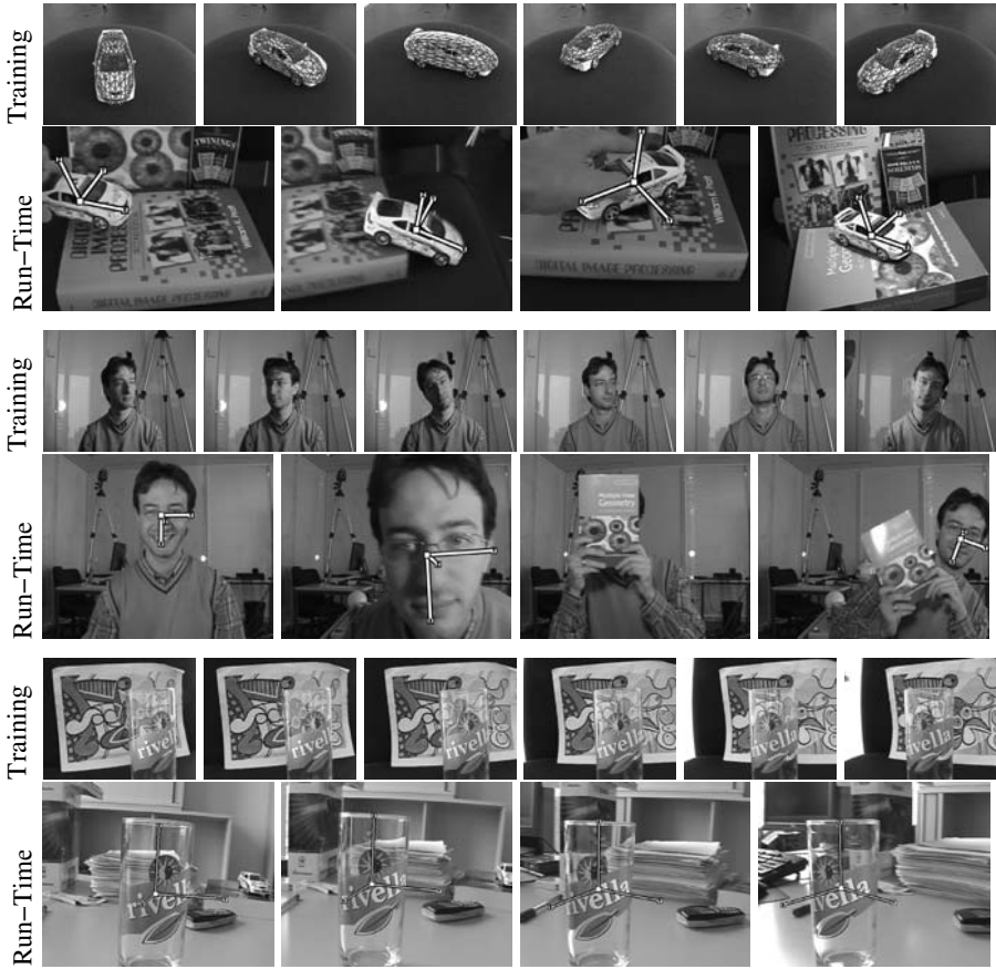
Fig. 1. Our approach to 3-D object detection applied to a toy car, a face, and a glass. In each one of the three cases, we show two rows of pictures. The first represents the training sequence, while the second depicts detection results in individual frames that are not part of the training sequence. We overlay the ellipsoid we use as our initial model on the images of the first row. The only required manual intervention is to position it in the very first image. To visualize the results, we attach a 3-D referential to the center of gravity of the ellipsoid and use the estimated 3-D pose to project it into the images. Note that, once trained, our system can handle large aspect, scale, and lighting changes. It can deal with the transparent glass as well as with the hand substantially occluding the car. And when a complete occlusion occurs, such as when the book completely hides the face, it simply returns no answer and recovers when the target object becomes visible again.
