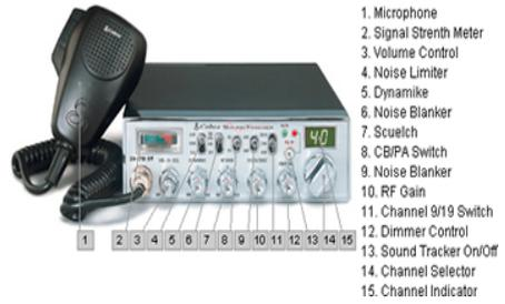
Fig. 2. A technical drawing of a cb radio
