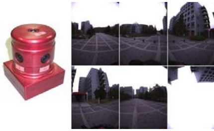
Fig. 4. Omni-directional camera system Ladybug and images taken by ladybug
