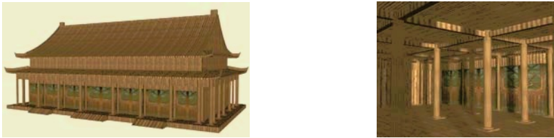
Fig. 5. Bamboo house. The control parameters of the model are 7AKR & 5AKC and the generating time is 0.381s. Left: the outside of the bamboo house; Right: the inside of the bamboo house
