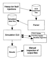
Figure 5. The basic work flow of the simulation tool environment
