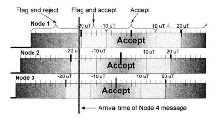
Figure 2. The modified receive window where node 4 is received early, too early by node 1
