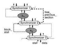
*Figure 3.* Synchronizer: A packet activates the *Block\_Stall* signal at  $N_2$ , that is transmitted to Synchronizier 2. This one generates a *Free\_Previous\_Section* signal and transmitted it to Synchronizier 1. Consequently section  $N_1$  is released.
