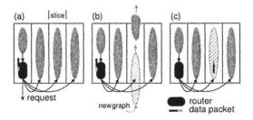
*Figure 6.* Reconfiguration: In situation (a) a packet reaches a router on an existing path stored in a slice. The router sends a *Request*-signal so that the slice is configured with a new operator network (b). Then the packet is routed to the network (c).
