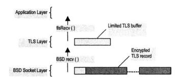
Figure 7. Reading a larger TLS record using a small TLS buffer
