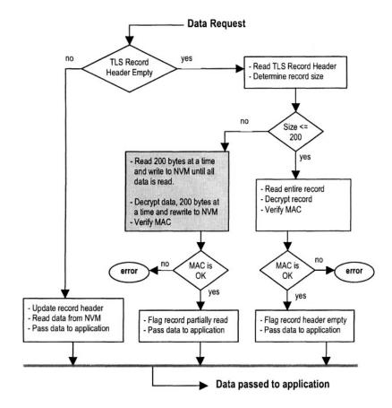
Figure 8. Error-critical design of reading TLS Record with limited I/O buffer.
