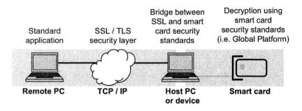
Figure 2. Bridging standard security layers in the host.
