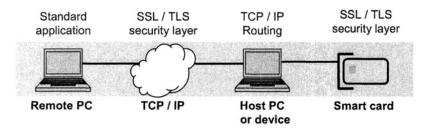
Figure 3. End-to-end security using SSL/TLS security within smart card.
