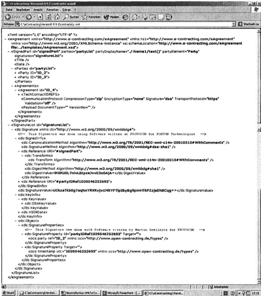
Figure 3: An XML document containing an electronic contract with a detached XML Signature
