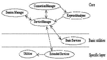
Figure 3. GenericServ based services providers' architecture.
