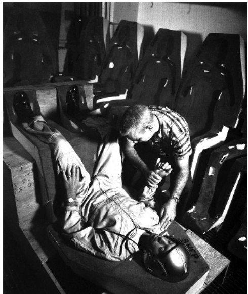
Figure 11-01. Contour couches were fitted for Mercury astronauts for performing physiological performance tests in the long-radius centrifuges. Flight versions of these couches were also used during spaceflight, for increasing tolerance to acceleration during launch and re-entry. Photo courtesy of NASA.
