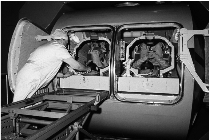
Figure 11-08. A technician reaches across the arm of a high-g centrifuge to prepare two subjects for a test run.
