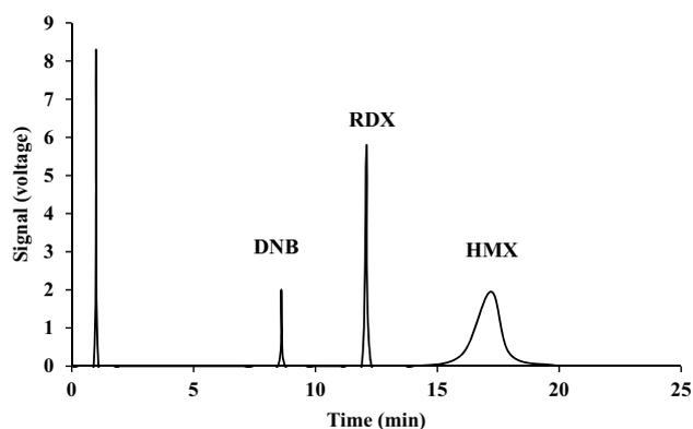
**Fig. 3** Chromatogram of a sample contains internal standard of DNB, 90 mg·L<sup>-1</sup> RDX in HMX matrix (0.12% W/V in acetonitrile solvent). The retention times were: DNB 8.6 min, RDX 12.1 min and HMX 17.2 min
