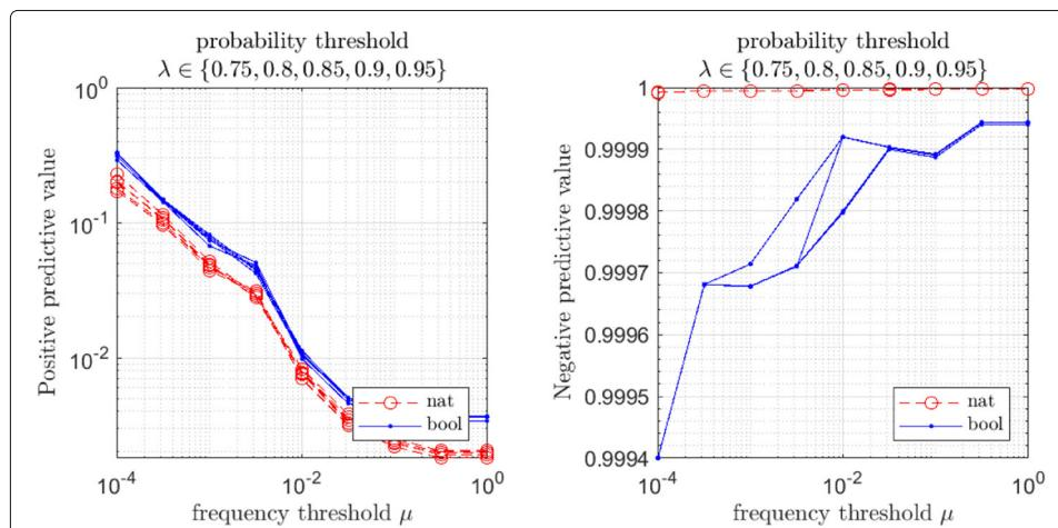
**Fig. 4** Positive (left) and negative (right) predictive values as defined in (11) for APT detections using the model of “Markov chain models for DCNs” section and as functions of a per-window frequency threshold  $\mu$  and for varying flow probability thresholds  $\lambda$
