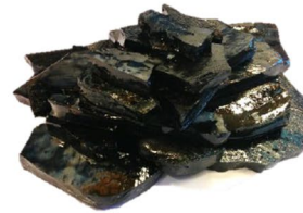
Vitreous blast furnace slag plates demonstrator sample, remolten BF slag
