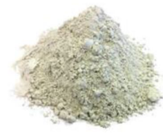
Granulated vitreous slag plates demonstrator sample, remolten BF slag
