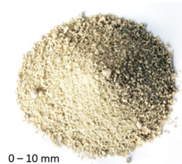
Granulated blast furnace slag industrial sample, GGBS
