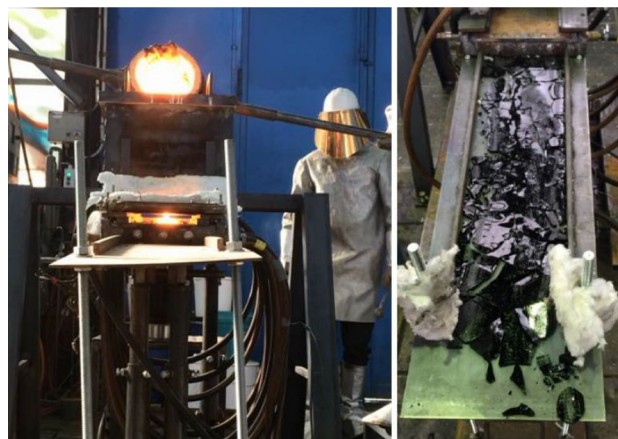
Fig. 3 Photograph of the first demonstrator during slag pouring in early stage (left) and vitreous solidified blast furnace slag after test and additional 30 min cooling at ambient air (right)
