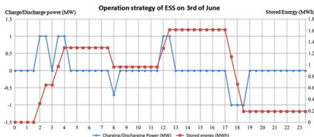
Fig. 7 The charging/discharging and power stored energy of BESS in the winter weekday (the blue line is the output power and the red line is stored energy)
