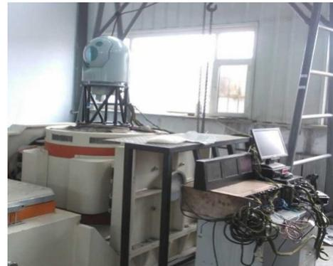
Fig. 2 Indoor test of the airborne PAT system.
