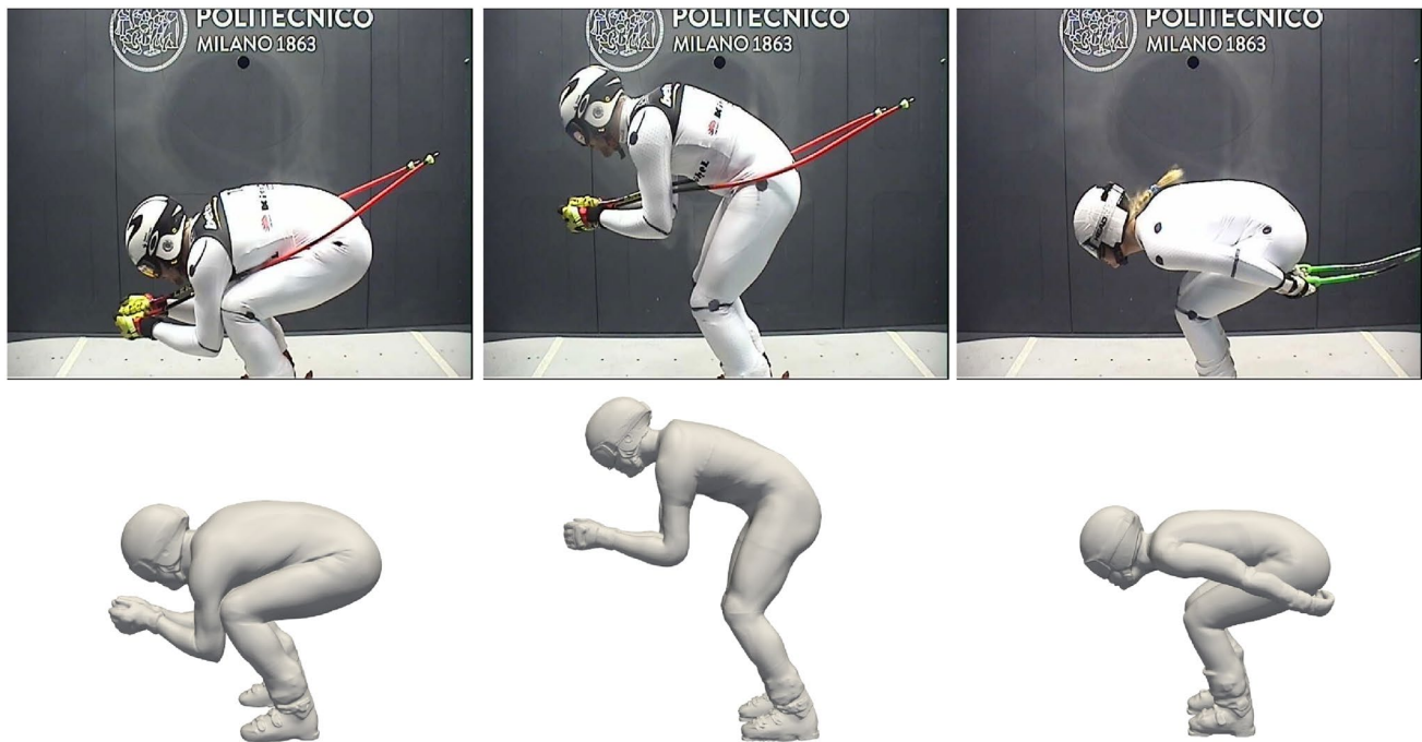
Fig. 1 Sample side-view images of the athletes in the wind tunnel (top) and the 3D model used in the simulations (bottom), showing low-tuck posture (left), high-tuck posture (middle), and flight posture with arms along torso (right)
