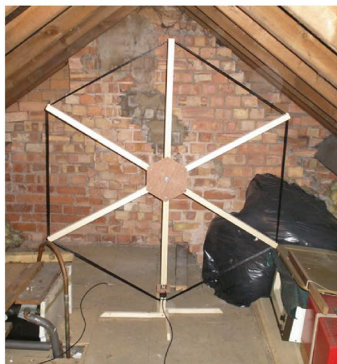
Fig. 5 The new antenna for the “SIDmonitor module” (left) and an example of acquisition on April 21, 2021 (right). Different curves in the right panels show different frequency bands (see text)
