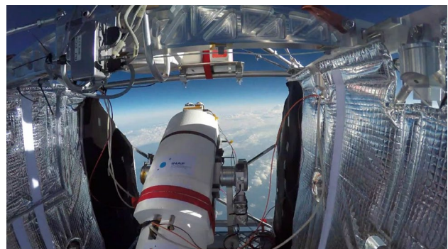
Fig. 14 CorMag coronagraph on the gondola operating at stratospheric altitude during the August 8, 2023 flight
