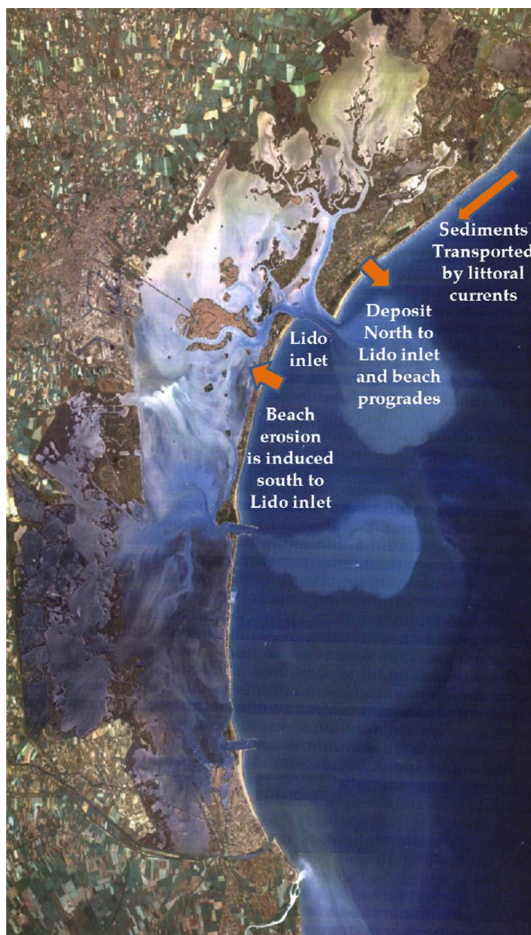
Fig. 25 Sketch illustrating the progradation of the coast north to the Lido inlet of Venice lagoon and the regression south to the same inlet
