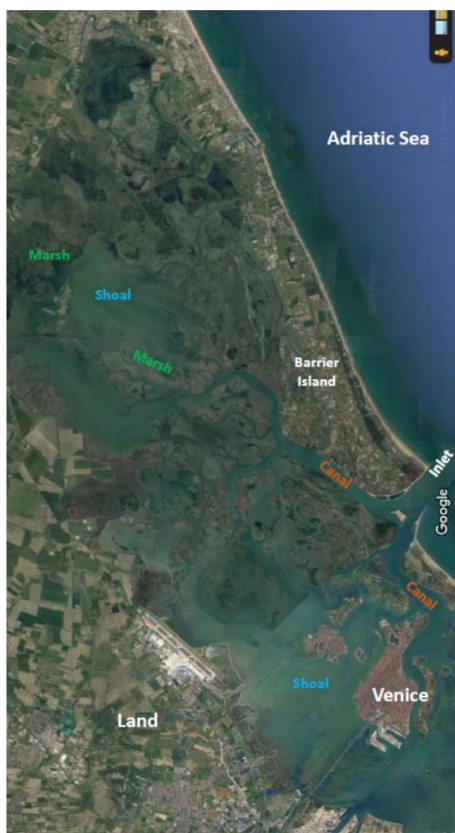
Fig. 4 Satellite view of the northern part of Venice lagoon, with indication of the various morphological features composing the lagoon environment. Note that in the Venice lagoon, sub-tidal flats and tidal flats are denoted as bassifondi and velme , respectively, while salt marshes are called barene
