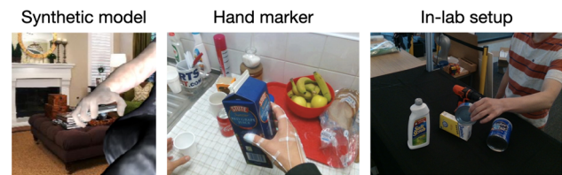
Fig. 4 Example of major data collection setups. The synthetic image on the left (ObMan (Hasson et al., 2019)) can be generated inexpensively, but they exhibit unrealistic hand texture. The hand markers on the middle (FPHA (Garcia-Hernando et al., 2018)) enable automatic tracking of hand joints, although the markers distort the appearance of hands. The in-lab setup on the right (DexYCB (Chao et al., 2021)) uses a black background to make it easier to recognize hands and objects, but it limits data variation in environments
