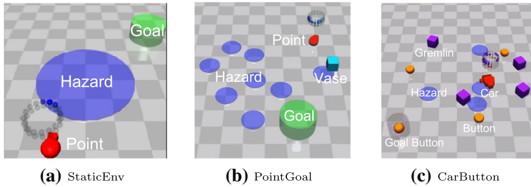
Fig. 8 Robot navigation environments. The three environments differ in complexity, i.e., the action space, the type of the obstacles, and the task. The Point or Car agent should avoid Hazards (dangerous areas), Vases (fragile objects), and Gremlins (moving objects) in the above environments, then move to the Goal position or press the Goal Button
