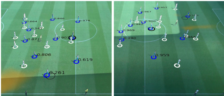
Fig. 10 Pass situations where real ball position and recorded data position differ significantly. Thick black circle indicates recorded ball position, light black circle indicates ball reception position. Orange shades indicate computed potential receiving positions. Left: The recorded ball position suggests that the ball is at the positions of the player’s heels. In reality, the ball is half a meter to the left. Computed availability indicates that according to recorded position the player at the bottom of the image can only receive a high pass to the left of him with probability 0.26. However, the real ball reception is at the light circle, following a low pass. Right: Recorded ball position is slightly below the player’s position. Real ball position is about a meter above the recorded position. For better visibility, a larger version of this figure is shown in Appendix C
