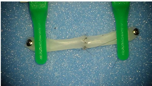
**Fig. 3** Robot-assisted anastomosis on 2-mm diameter silicone vessel [15]
