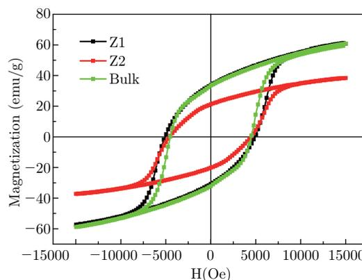
Fig. 5 Magnetic field vs. magnetization plots Z1, Z2 and bulk BaFe<sub>12</sub>O<sub>19</sub> (unmodified).
