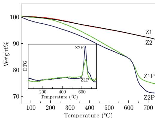
Fig. 4 TGA thermograms of precursor (Z2p, Z1p) and calcined (Z2, Z1) hexaferrite powders.
