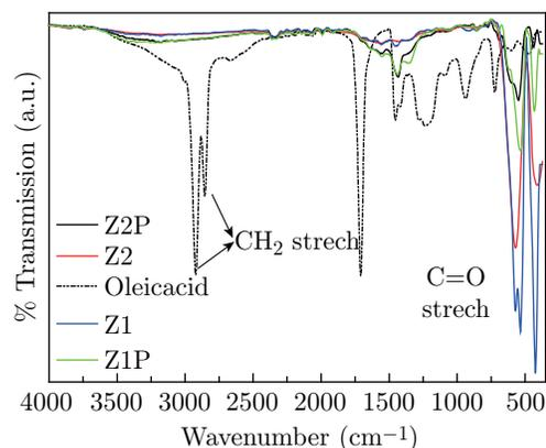
Fig. 2 FT-IR spectra of the dried precursors (Z1p, and Z2p), oleic acid and precursors calcined at  $1100^{\circ}\text{C}$  for 1 h (Z1 and Z2).
