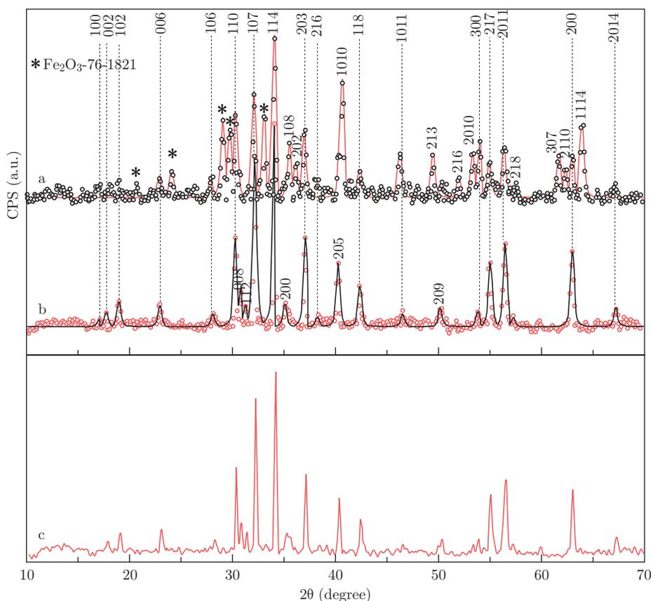
Fig. 3 XRD powder patterns and line profile fittings of: (a) Z1; and (b) Z2; and (c) bulk  $\text{BaFe}_{12}\text{O}_{19}$ .
