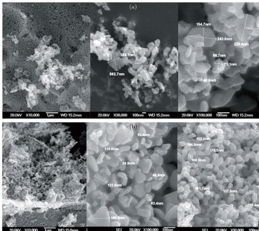
Fig. 1 SEM images of: (a) Z1 at different magnifications; and (b) Z2 at different magnifications.
