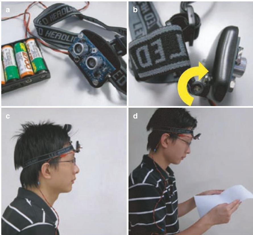
**Fig. 7.7** Front view (a) and side view (b) of the near work analyzer for logging near work distance and its alignment in a straight-ahead position (c) and reading position (d). © Leung et al. [57]
