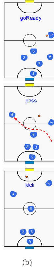
Fig. 11. An example of indirect free kick in frontcourt: (a)Lua script; (b)positions of robots in every state. In the script (a), the basic settings are from line 1 to line 4. Then we define the specific states in this play. For example, the state goReady comprises a role match item (line 6), switch condition (line 7-9) and execution (line 10-12).
