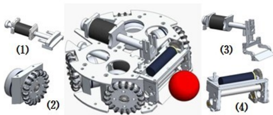
Fig. 1. Mechanical design of the robot: (1)shooting device; (2)omni-directional wheel; (3)chipping device; (4)dribbling device
