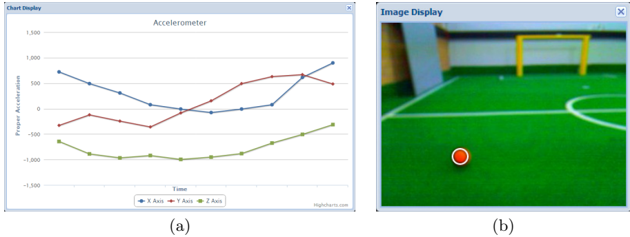
Fig. 4. Two examples of NUbuzzer debugging interfaces: a) the scrolling chart display, demonstrating real-time information from the robot’s 3-axis accelerometer; and b) the image display, with an overlay demonstrating the correct identification of the ball [2].
