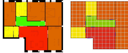
Fig. 1. An example of a floor plan of a house made with AutoCAD (left) and with our CAD-like software (right). Colors indicate semantic labels (green is corridor, yellow is small room, red is big room, brown is medium room).
