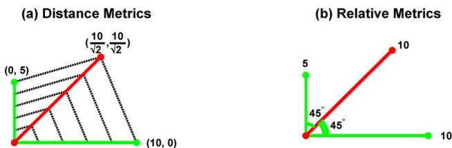
**Fig. 3.** Deciding which candidate hallway (green) to snap the trajectory update (red). A distance metric would select the shorter hallway because the sum of sampled distances (dashed) is smaller. The relative metric separates rotation and motion errors and selects the longer hallway because it only differs from the trajectory update by rotational error while the shorter hallway differs by both rotational and motion errors.
