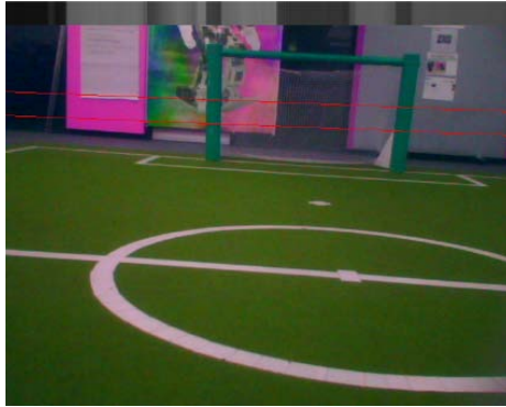
Fig. 1. Image captured by the Nao robot showing superimposed 30 pixel horizon band in red, and the extracted grey-scale horizon pixels used for 1D SURF feature extraction at the top of the image
