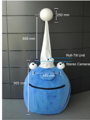
**Fig. 1.** The developed robot system, its major components, and dimensions. The computer and the motor's power supply are inside the robot's body.
