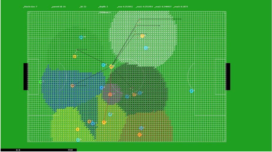
Fig. 4. Red lines mean the passes in history, black lines mean the considering passes. Different colors represent different teammates' control areas.
