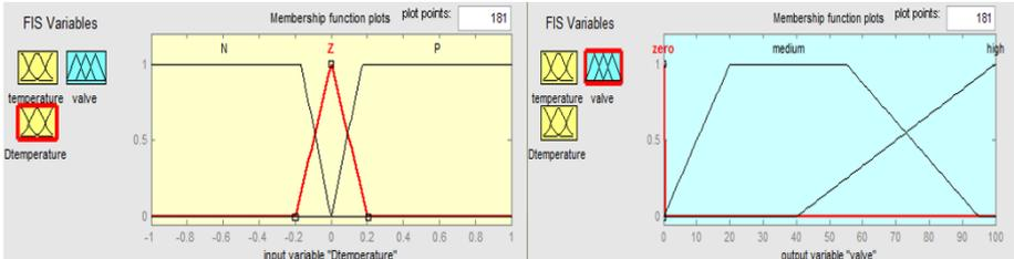
Fig. 4. and Fig. 5. Membership functions to temperature derivative and percentage of valve opening
