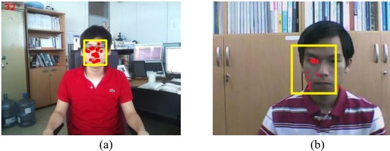
**Fig. 2.** Feature tracking. (a) extracted corners in the face region (b) the divergence problem.
