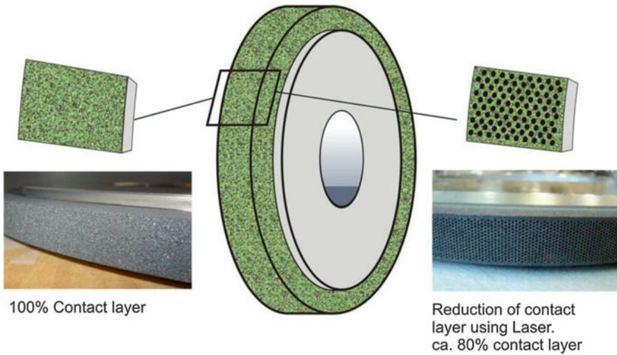
**Grinding Tool Structuring, Fig. 4** Nd:YAG laser structured wheel surface from (Rabiey 2010)
