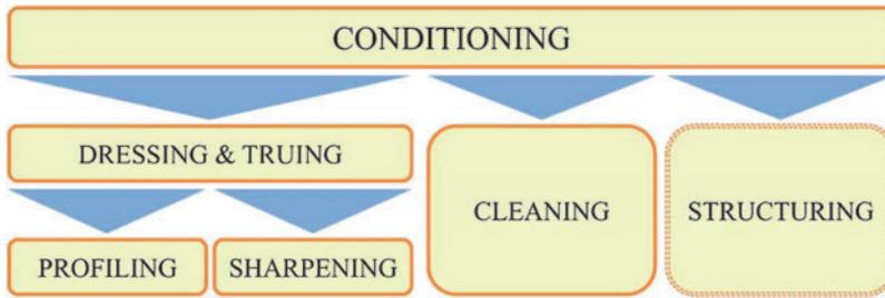
**Grinding Tool Structuring, Fig. 1** Classification of grinding wheel conditioning processes according to VDI guideline 3392 (2007), complemented by structuring as an additional process according to Walter et al. (2014)
