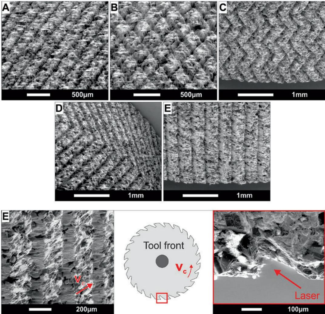
**Grinding Tool Structuring, Fig. 6** Different patterns from laser structuring of hybrid bonded CBN grinding wheels. Especially pattern E shows that also cutting edges may be shaped by structuring (Walter 2014)
