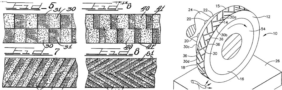
**Grinding Tool Structuring, Fig. 2** Grooved wheel geometries proposed by Sherk (1936) (left) and deGraaff (1997) (right)
