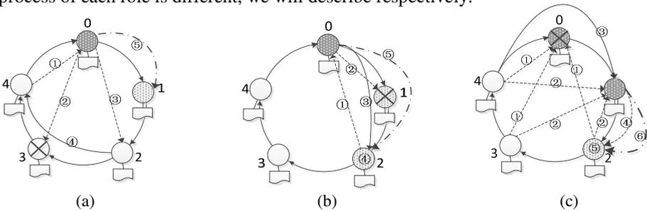
Fig. 3. Node Failure Detection Process. (a) Common node failure detection process. (b) Backup node failure detection process. (c) Leader node failure detection process.
