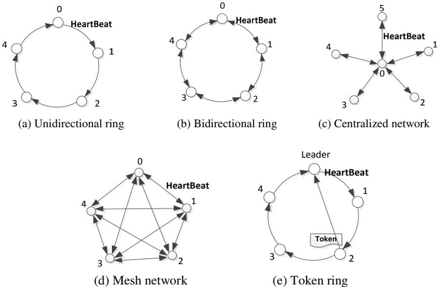
Fig. 1. Classical node failure detection models
