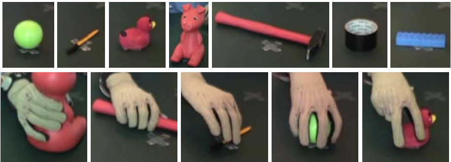
Fig. 3. Top row: the objects used in our experiments. Bottom, the grasp types we consider: (left to right) cylindrical power grasp, flat grasp, pinch grip, spherical and tripod grasp.
