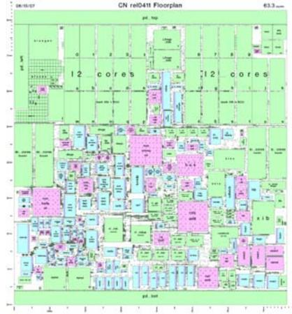
**Fig. 2.** Floor Plan of Centaur CN
