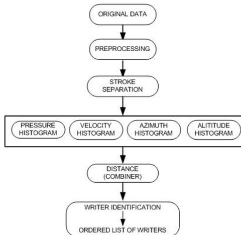
Fig. 1. Schematic diagram of the proposed algorithm
