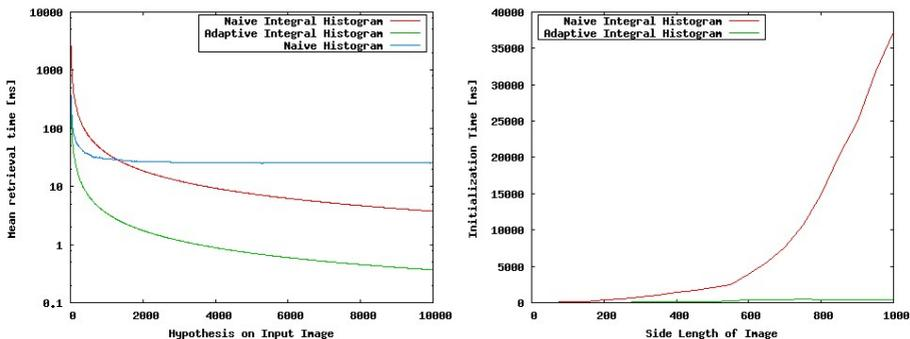
**Fig. 3.** Left: Mean retrieval times (note the logarithmic scale), Right: Initialization times subject to side length of the input image
