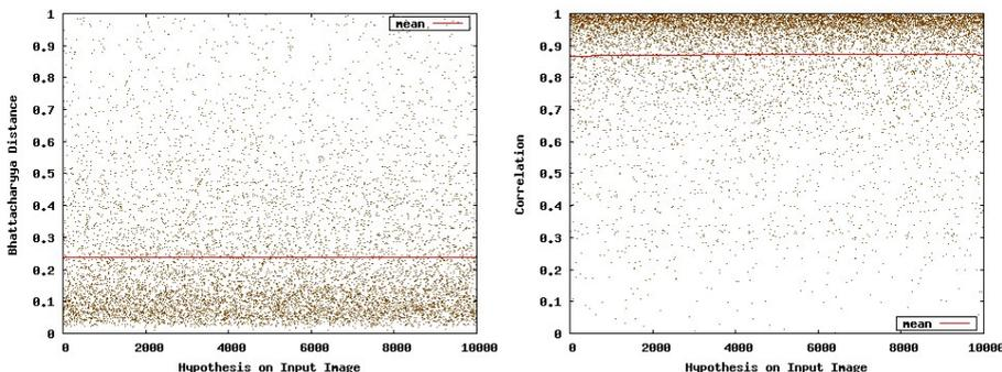
**Fig. 4.** Accuracy using the adaptive integral histogram approach compared to exact solutions (left: Bhattacharyya Distance, right: Correlation) on random patches
