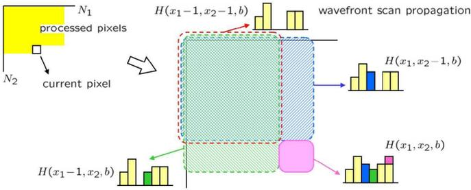
**Fig. 1.** Propagation of integral histogram by wavefront scan<sup>1</sup>
